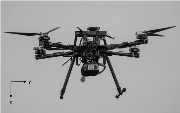
Figure 2: Photograph of the experimental UAS platform used in the experiments. The vehicle appears equipped with a set of asymmetric propellers.
