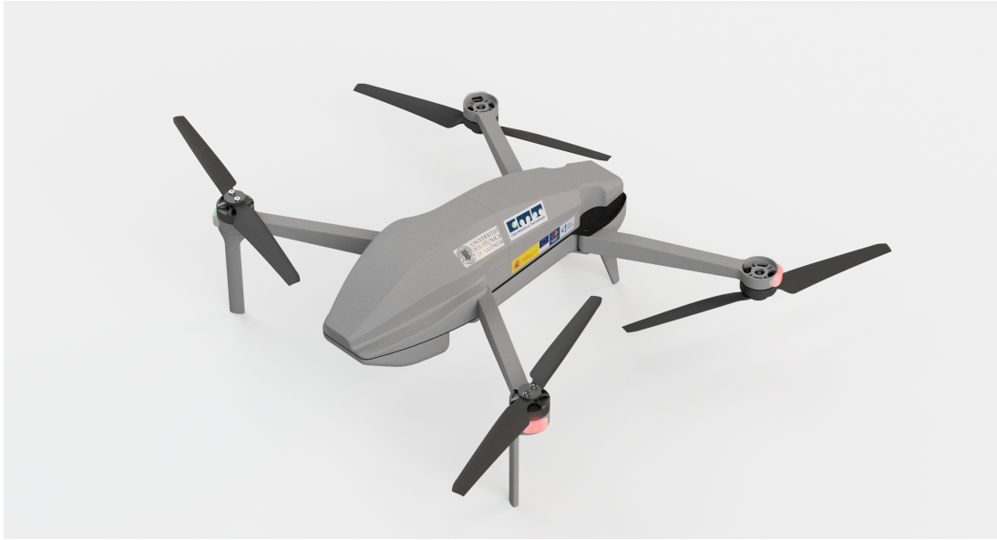
Figure 1: Render of the Hunter quad-rotor Unmanned Aerial Vehicle manufactured by UAV-Works.
