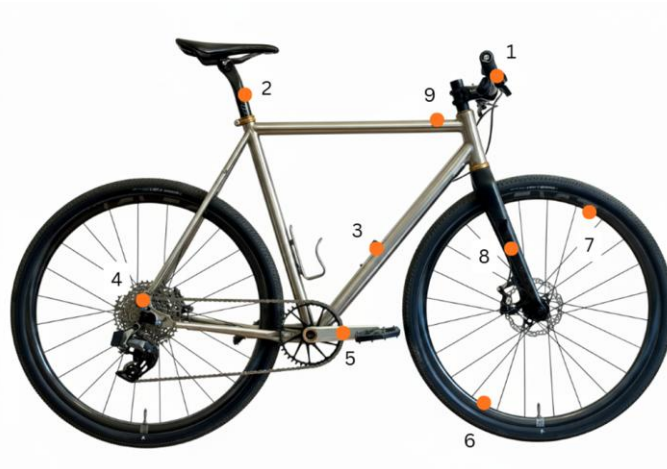
Figure 2: Test bicycle measurement points: 1. Handlebar; 2. Seat post; 3. Frame down tube; 4. Rear drop down tube 5. Pedal; 6 and 7: Wheel; 8. Fork and 9. Frame.
